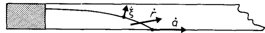
Figure 7 Diagram showing the three different speeds considered for the description of crack propagation.
